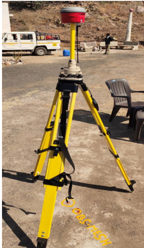
Figure 5.3-1 DGPS Observation at Dam top
