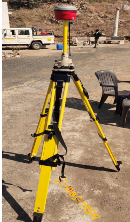
RTK Observation At Dam Top
